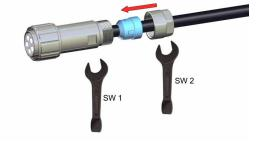
Insert sealing (3) completely and screw cap (2) onto basis (5).
