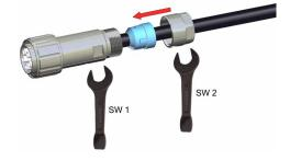
Insert sealing (3) completely and screw cap (2) onto basis (5).
