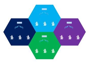
The CBRS topology is modeled after the cellular architecture. The SAS assigns non-overlapping/non-interfering channels to the adjacent cells. This greatly increases the ability to deploy large private networks without the worry of interference.
