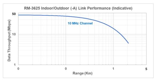
CBSD-A Antenna = 6 dBi, EUD Antenna = 3 dBi, PtmP configuration Fade Margin = 10 dBm, Fresnel Zone 60% Clearance
