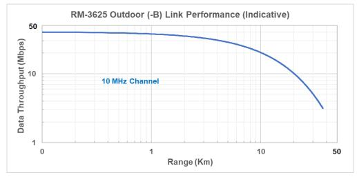
CBSD-B to CBSD-B for PtP configuration. Antenna = 17 dBi Fade Margin = 20 dBm, Fresnel Zone 60% Clearance
