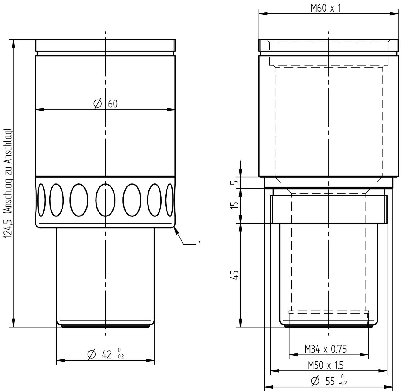
\*: clamping ring (for mounting plate with dia. 55 through hole, thickness max. 10)
