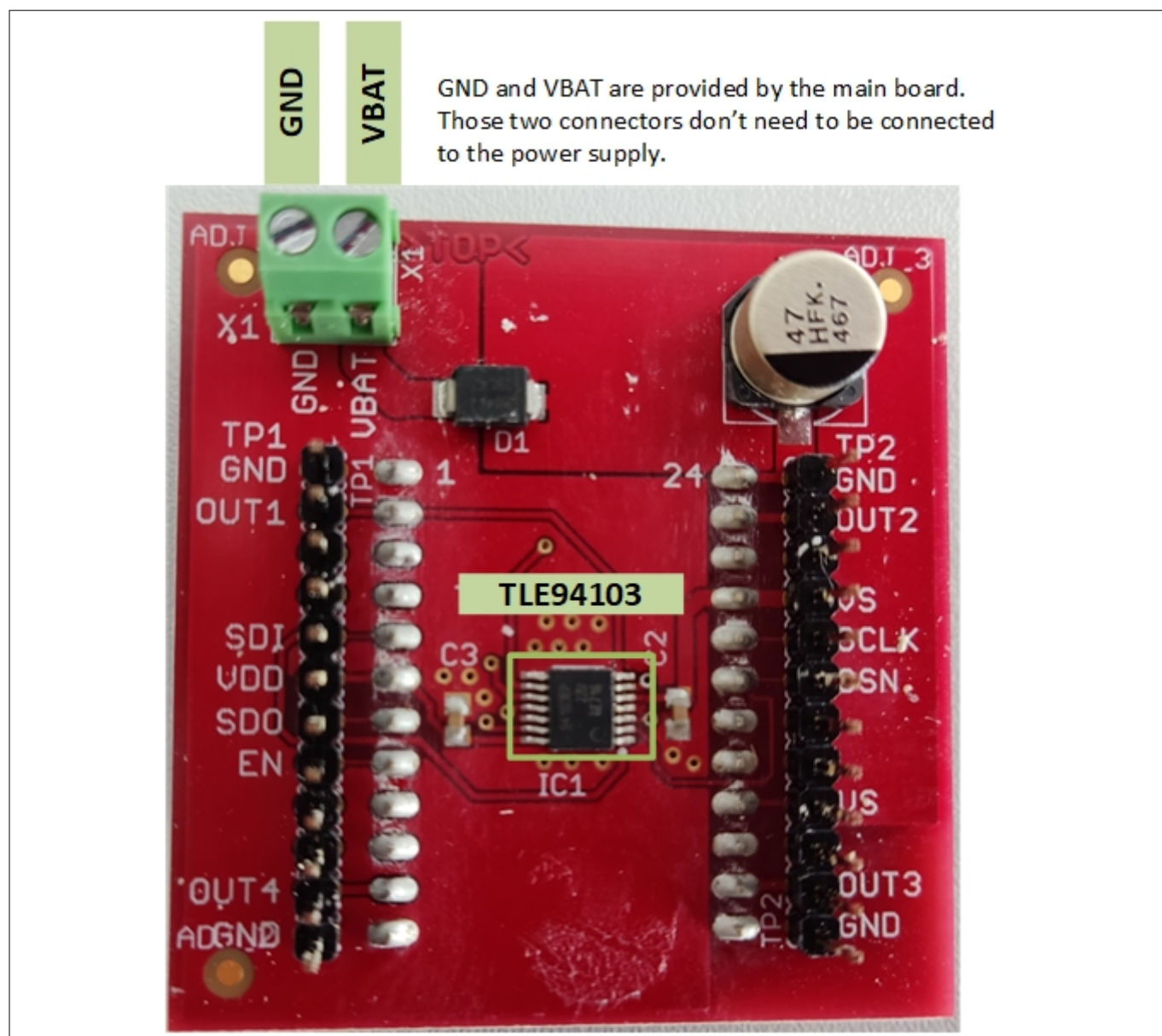
Figure 9 TLE94103 evaluation board – daughter board
