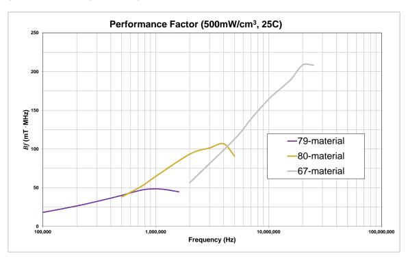
Fair-Rite's **79-material** product line continues to expand and include new geometries for power supply designs. With operating frequencies up to **1 MHz**, this material is optimized for minimal losses at elevated temperatures.
