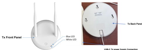
Figure 3: Energos 1W Omnidirectional PowerBridge Transmitter
