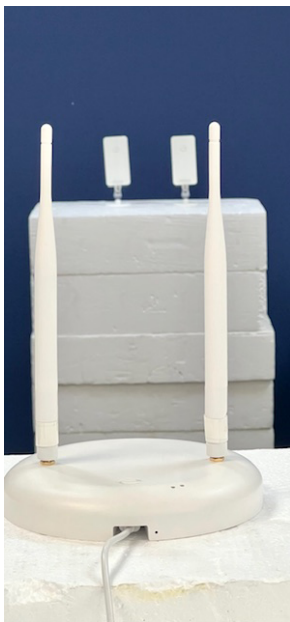
Figure 5: Energous 1W Omnidirectional PowerBridge Transmitter and Receivers
