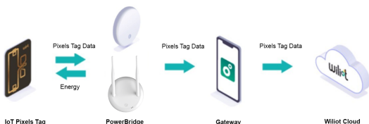
Figure 1: Wireless Power Network System Diagram
