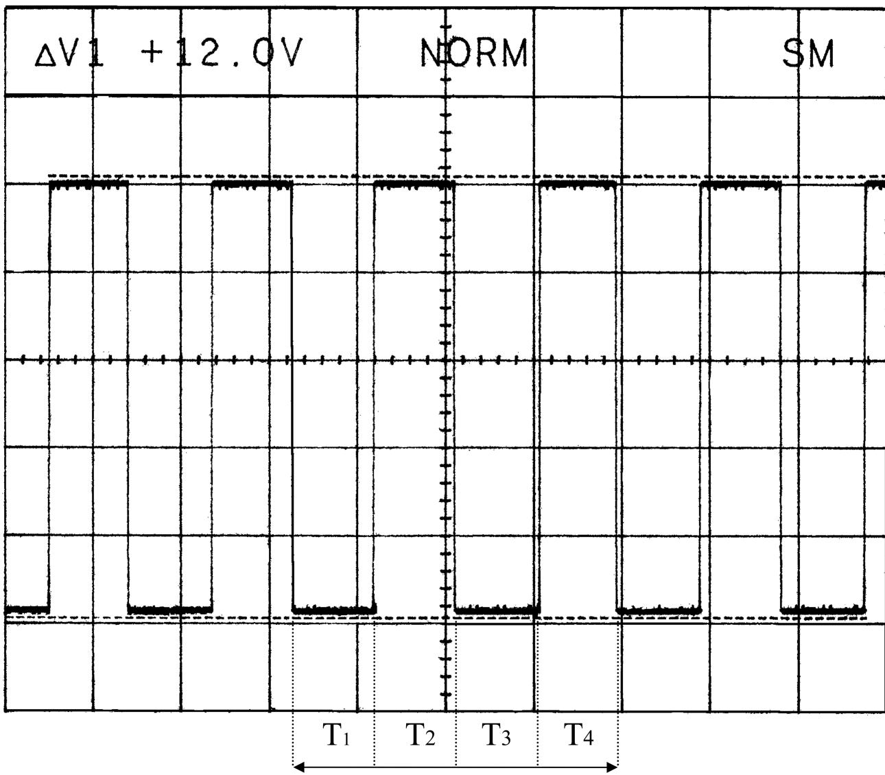
$$T = T_1 + T_2 + T_3 + T_4 = (1 \text{ Rotation})$$
