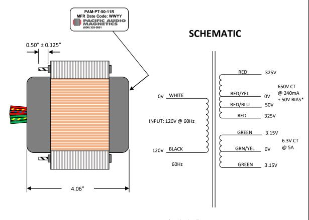
\*Vct (no-load): 335V – 0V – 335V Vct (simulated): 325V – 0V – 325V
