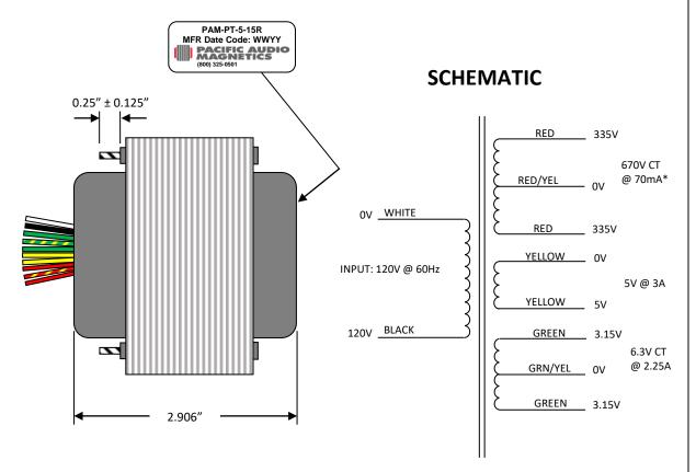
\*Vct (no-load): 365V – 0V – 365V Vct (simulated): 335V – 0V – 335V
