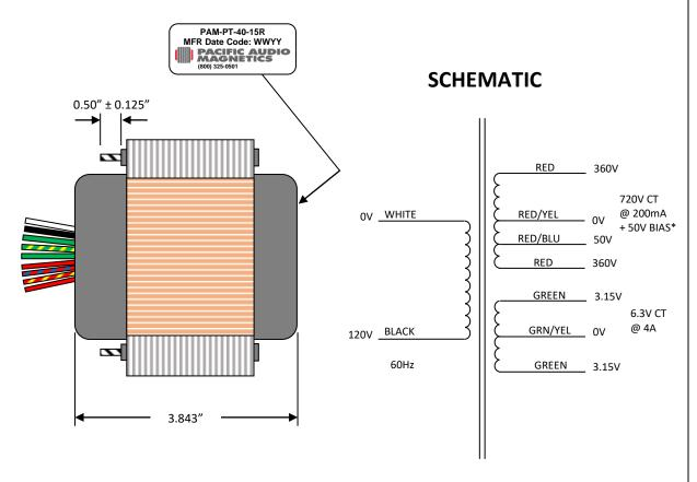
\*Vct (no-load): 380V – 0V – 380V Vct (simulated): 360V – 0V – 360V
