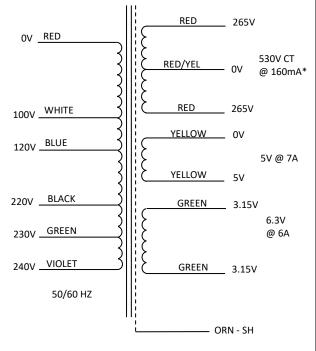
\*Vct (no-load): 280V – 0V – 280V Vct (simulated): 265V – 0V – 265V
