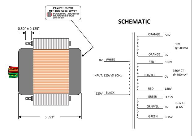
\*Vct (no-load): 185V – 0V – 185V Vct (simulated): 180V – 0V – 180V
