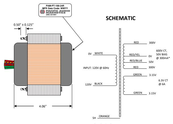
\*Vct (no-load): 315V – 0V – 315V Vct (simulated): 300V – 0V – 300V
