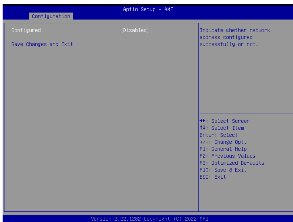
Figure 6-8 “Ethernet port Configuration” screen showing Disabled options
