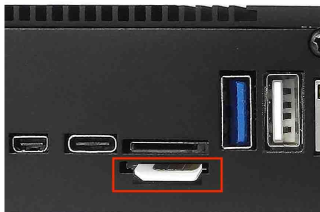
SIM Card Direction (Micro SIM Card)
