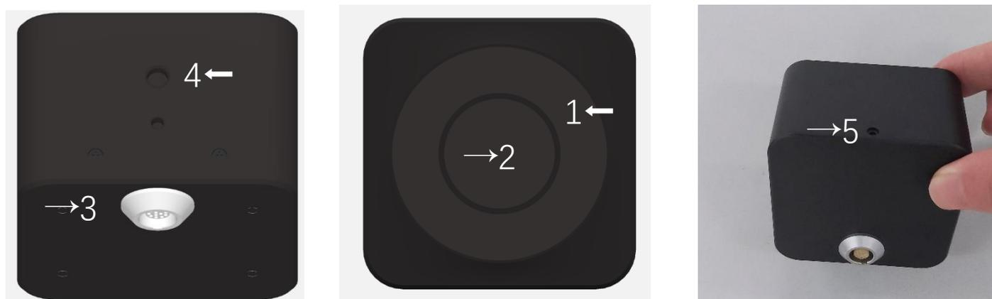
1. Big baffle Vcsel launch window, light through the window for launch, detect the objects within FOV range.
