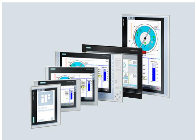
SIMATIC Panel PCs are suitable thanks to their high industrial compatibility for use in control cabinets, consoles and control panels, as well as directly on the machine. Typical areas of application can be found in both factory and process automation.
