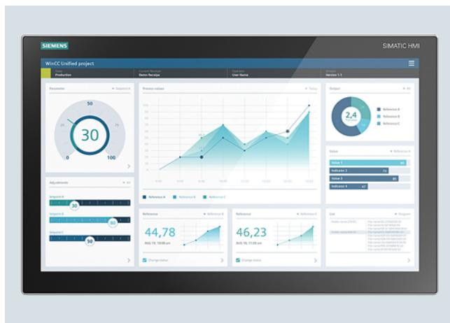
SIMATIC HMI MTP2200 Unified Comfort Panel Standard design front view
