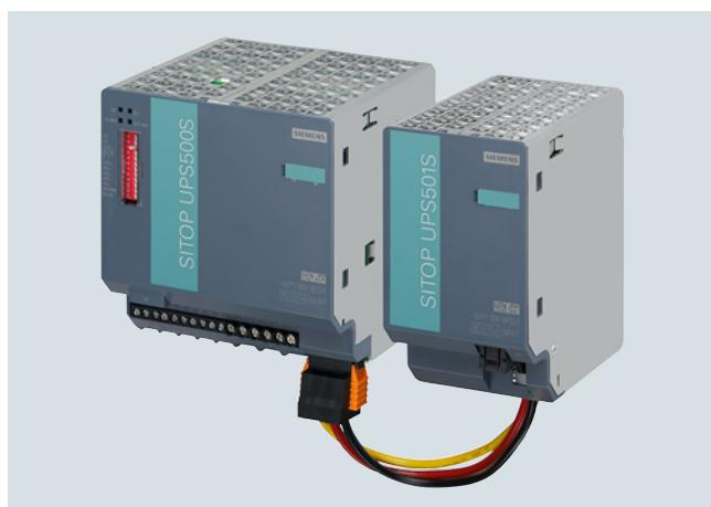
SITOP 24 V power supplies can be expanded with a SITOP UPS500 uninterruptible DC power supply (DC UPS) for bridging short-term power failures in the order of minutes. In PC-based automation solutions, the highly capacitive double-layer capacitors of the SITOP UPS500 supply enough energy to safeguard operating and application data and close software applications in a defined manner. You can increase the buffer times using SITOP PSU501S expansion modules (up to 3).
