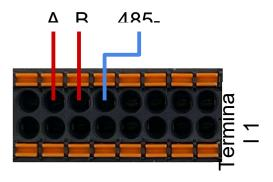
RS485 can work by only connecting the A-B signal. However, we do also recommend connecting the GND too for better noise immunity.
