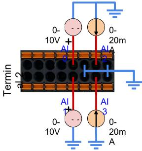
⚠ The AGND is isolated from the system ground, but it's common among all the analog input channels.
