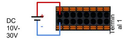
The power supply input is fuse protected. The fuse might break in the event of surge or overcurrent. If the device is unable to power up, check the 4 Amp fuse and replace it if needed.
