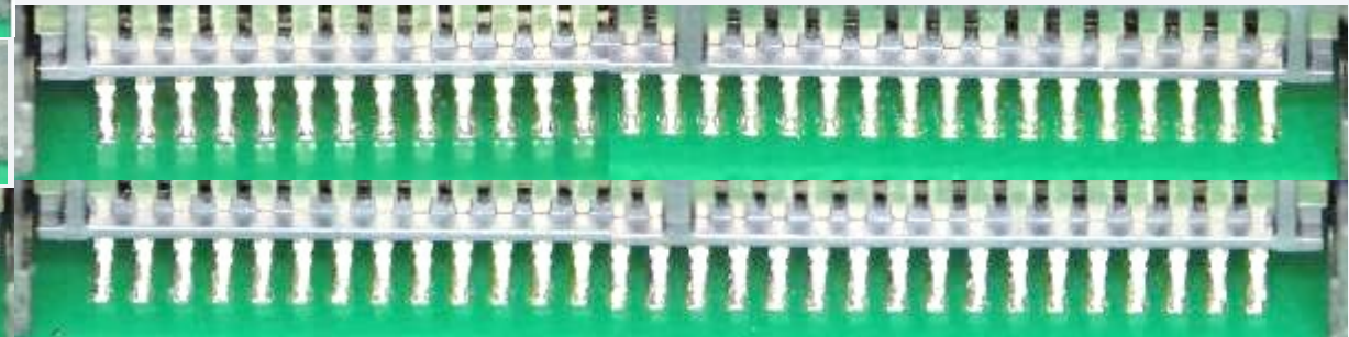
Sample pictures of solder tail after first re-flow (260°C)
