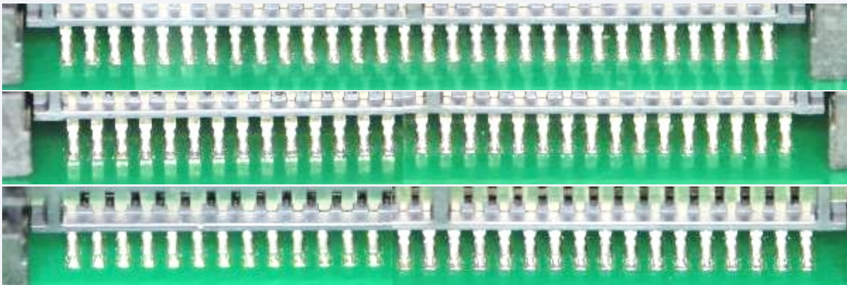
Sample pictures of solder tail after first re-flow (260°C)
