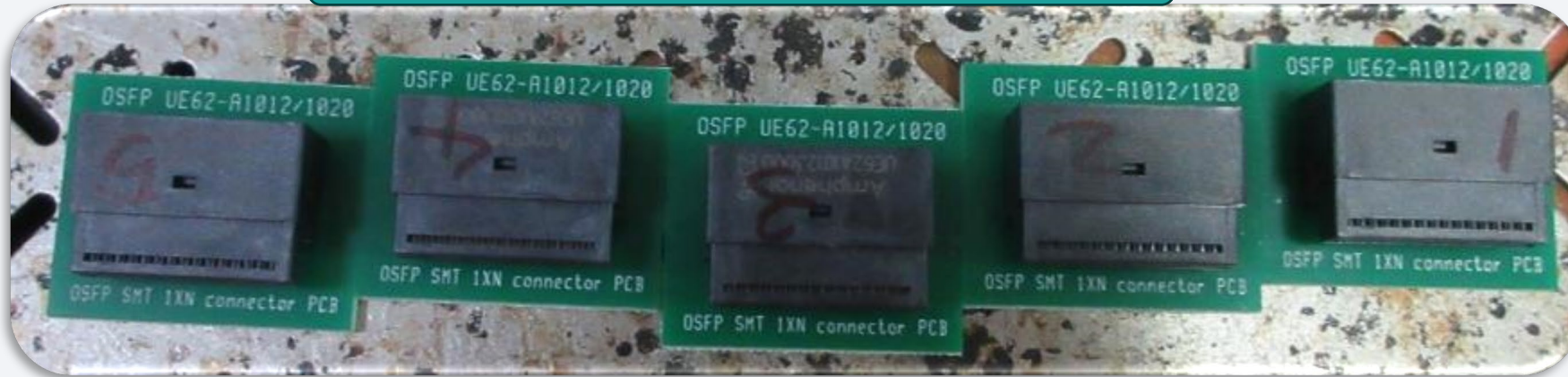
Sample pictures for the first re-flow (260°C)
