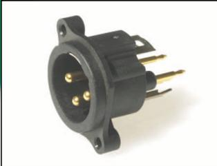
**XNACM2V / PCS 3 Pin vertical PCB mounting Male XLR with non counter sunk mounting holes for self-tap screw fixing. Gold plated Brass contacts standard.**
