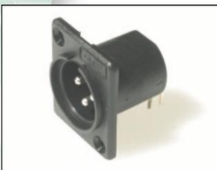
**ACM / PC 3 Pin horizontal PCB mounting Male XLR with counter sunk mounting holes for M3 screw fixing. XACM / PC has non counter sunk mounting holes for self-tap screw fixing. Nickel Silver plated Brass contacts.**
