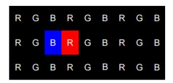
**Two adjacent dots (vertical direction):** Use the bright spot illustration as an example to demonstrate two vertical consecutive dots.
