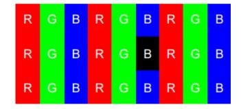
**Two adjacent dots (horizontal direction):** Use the bright dot illustration as an example to demonstrate two horizontal consecutive dots.
