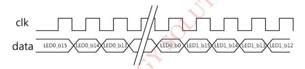
Data is to be transmitted on the rising edge of CLK MSB first starting at LED0; see scan direction reference below. Data must be transmitted for all LEDs for the panel to update brightness. To reject data prior to completing transmission, resend the start transmission condition.
