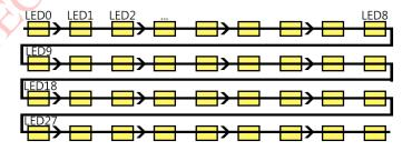
LED0 is in the upper left corner of the screen. LEDs increment left to right and continue incrementing on the left LED of the row below.
