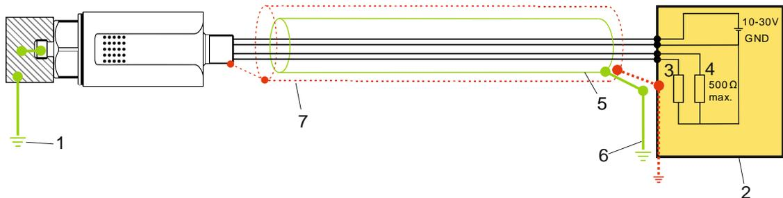
Fig. 10: Standard earthing concept
