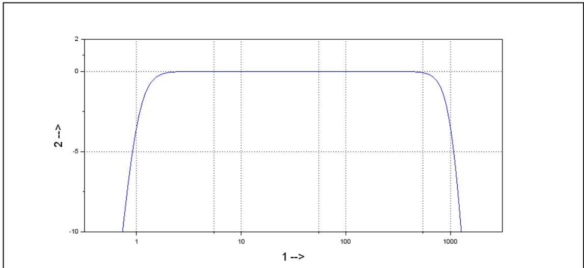
Fig. 7: Typical frequency response 1 Hz–1000 Hz
