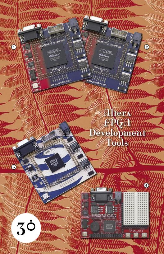
The Stratix™ and Cyclone™ SmartPacks and FastPack make it easy for you to explore powerful FPGAs from Altera®. FPGAs are reconfigurable logic chips which contain many thousands of gates. If you've ever wanted to break beyond the constraints imposed by microcontrollers and make your own systems instead, this is what you need. These FPGA boards are for advanced customers and are not related to the BASIC Stamp microcontroller line of products.
