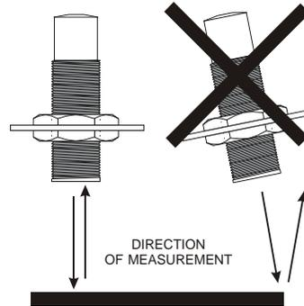
Figure 4 - Sensor Orientation
