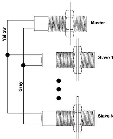
Figure 24 - SYNC Wiring
