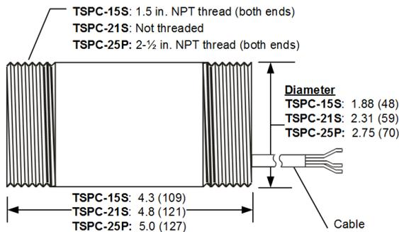
Figure 3 - Mechanical Drawing, ToughSonic 30, 50, and 50P
