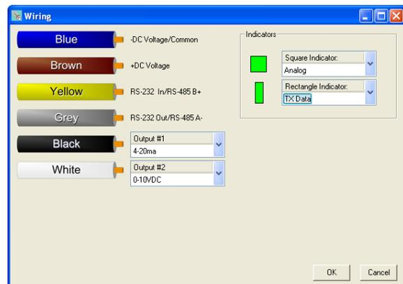
For ToughSonic 30, 50, and 50P sensors the following 9-wire dialog appears. Note that each output has a separate wire in these models.
