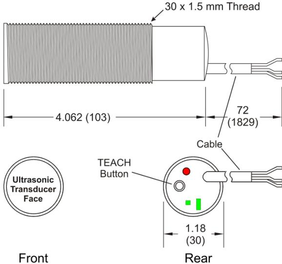
Figure 2 - Mechanical Drawing, ToughSonic 3, 12, 14 metric thread
