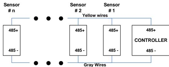
Figure 21 - RS-485 Network Wiring
