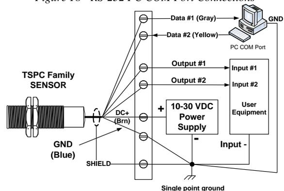
Figure 19 - RS-232 Connections
