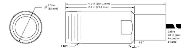
Mechanical Drawing, ToughSonic 3, 12, & 14 NPT thread
