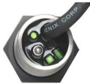
Some models utilize a rear TEACH button to make many common adjustments. See the Teach Adjust section. Rear indicators provide target and output status. The TEACH button can be disabled for security
