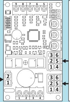
Molex 6-pin connectors with same connection for both actuator and control.
