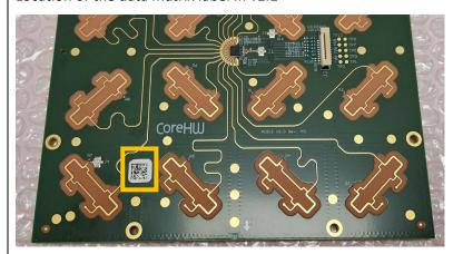
Data matrix code can be read to verify whether the antenna version is 1.0 ( A2-1010-**1.0**-XYZ... ) or 1.1 ( A2-1010-**1.1**-XYZ...)
