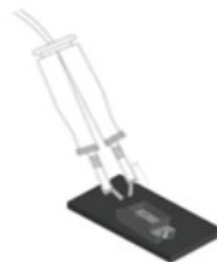
Fig2. Repairing using a double-head soldering iron
