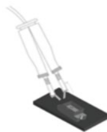
Fig2. Repairing using a double-head soldering iron
