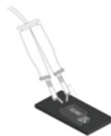
Fig2. Repairing using a double-head soldering iron
