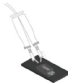
Fig2. Repairing using a double-head soldering iron
