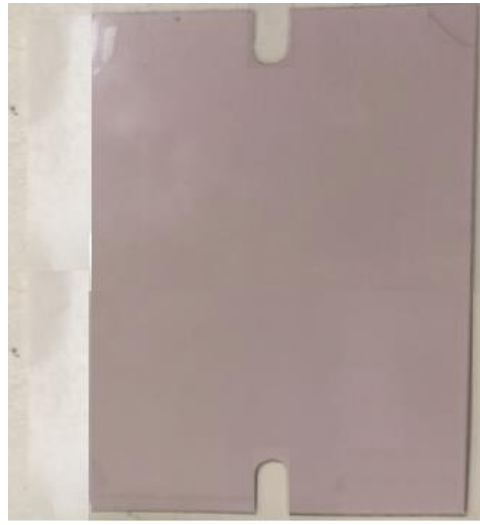
Thermal Pad with Alternative Material
