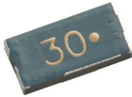
The XRA30AA30SES is a high performance Aluminum Nitride (AlN) chip attenuator intended as a cost competitive alternative to Beryllium Oxide (BeO). It is designed particularly for LTE and 5G wireless communication frequency bands. The high power handling makes the part ideal for inter-stage matching, directional couplers, and for use in isolators. The attenuator is also RoHS compliant!
