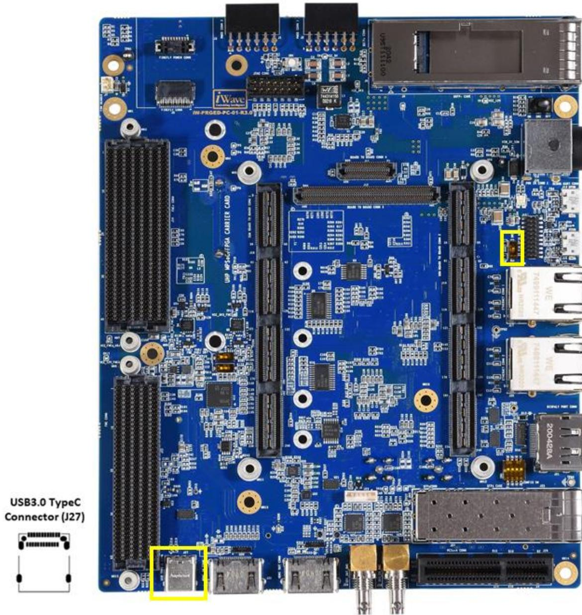
Figure 14: USB Type-C Connector
