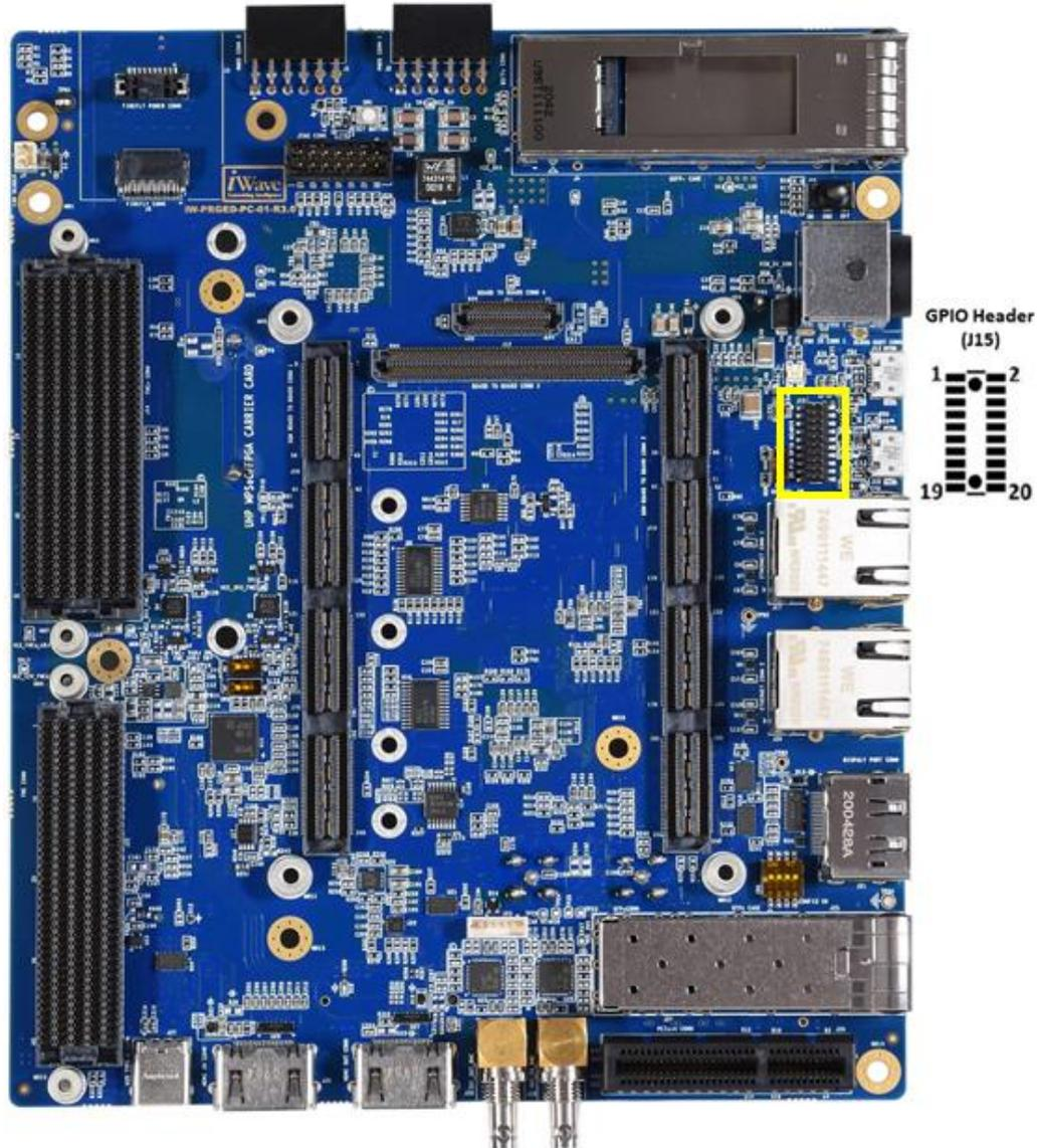
Figure 30: GPIO Header
