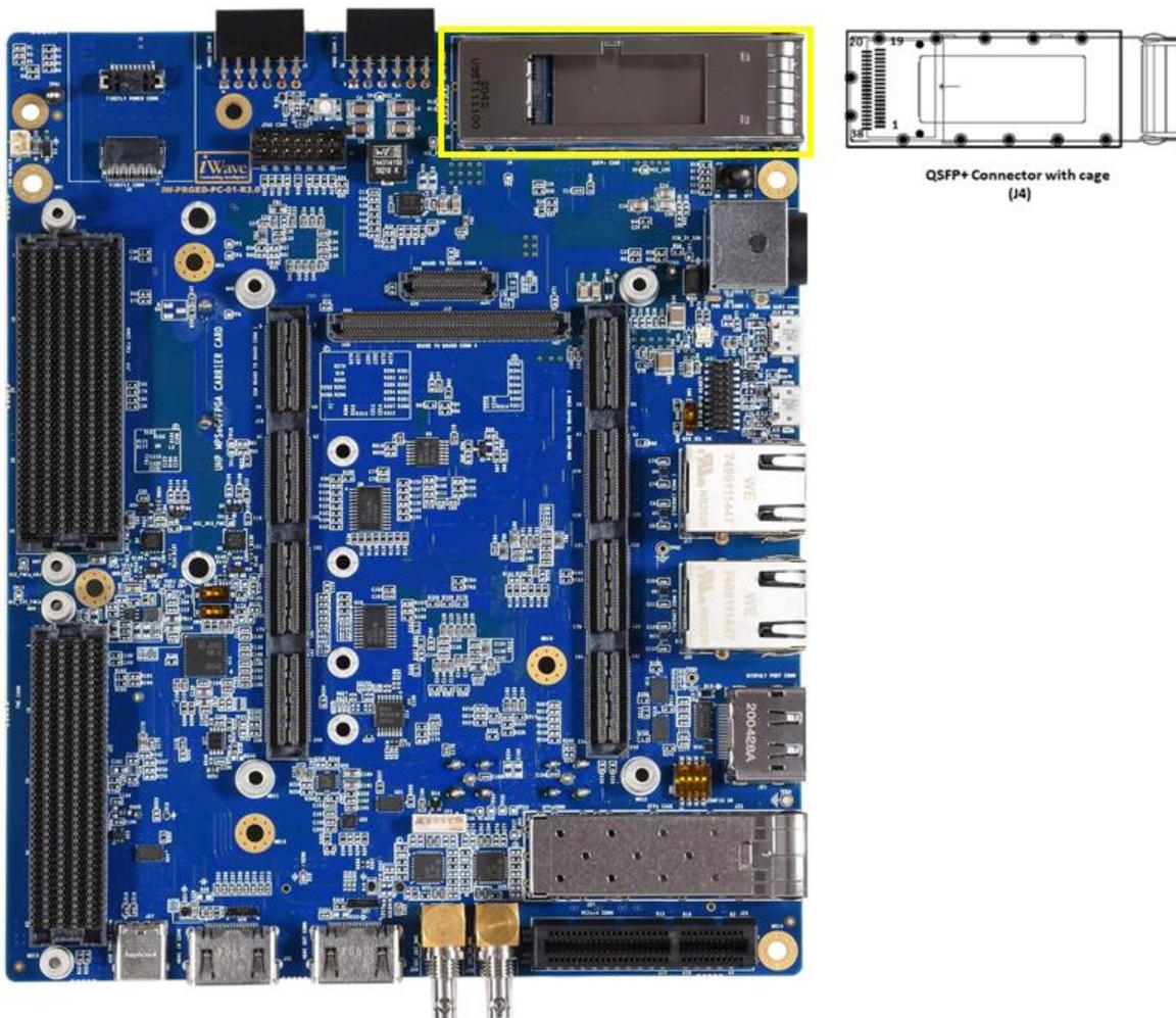
Figure 19 QSFP28/QSFP+/QSFP+ Connector with Cage
