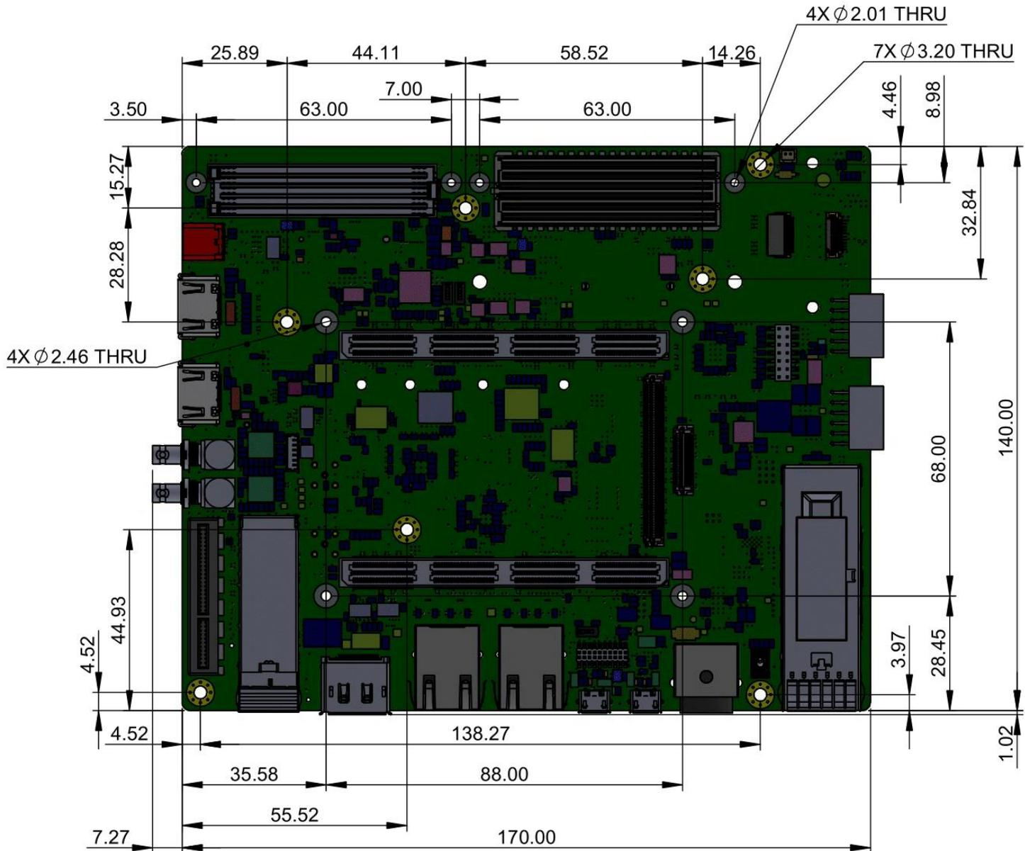
Figure 36: Carrier board Mechanical dimension – Top View
