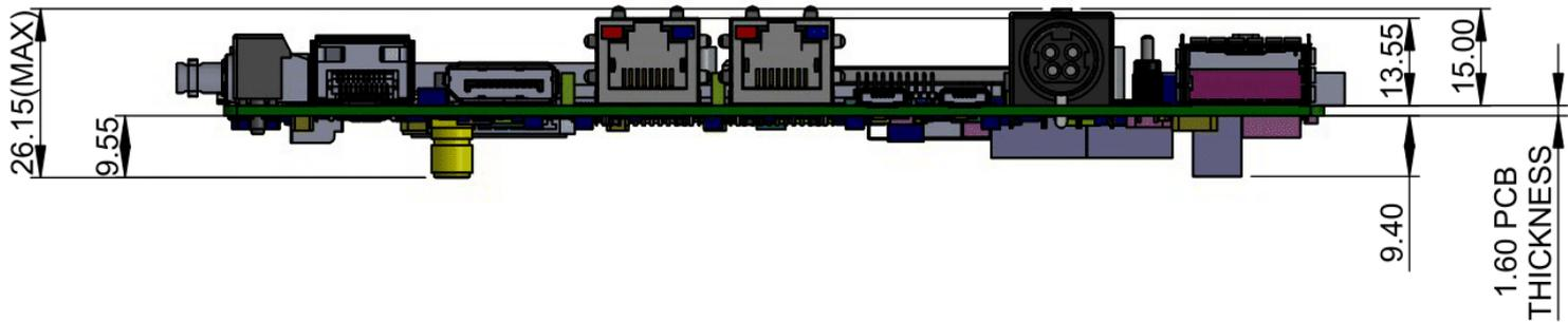
**Figure 37: Carrier board Mechanical dimension – Side View**
