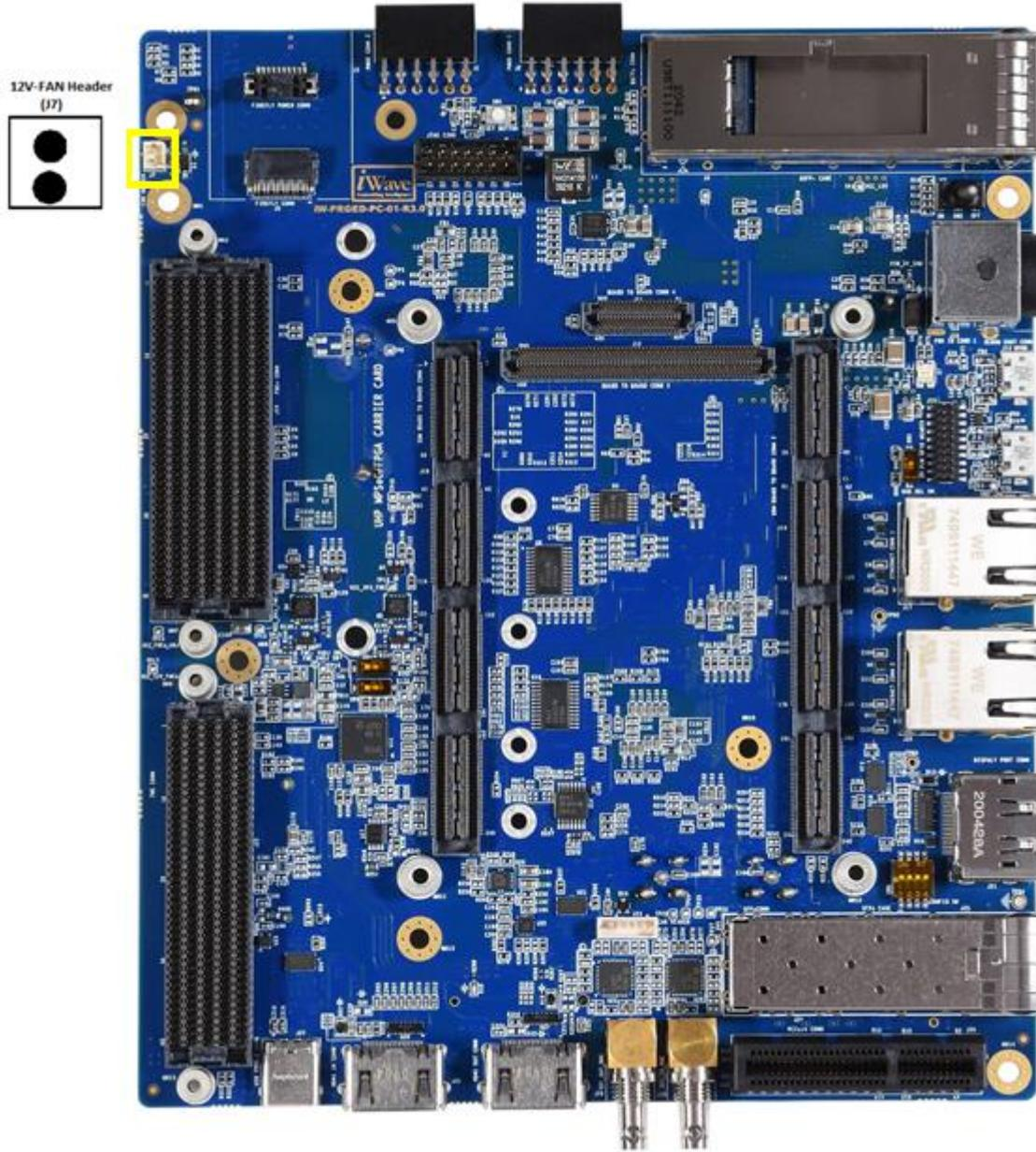
Figure 34: 12V-Fan Header
