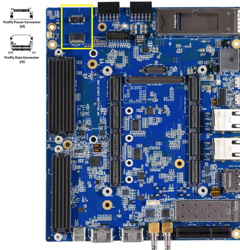
Figure 20 FireFly Connector
