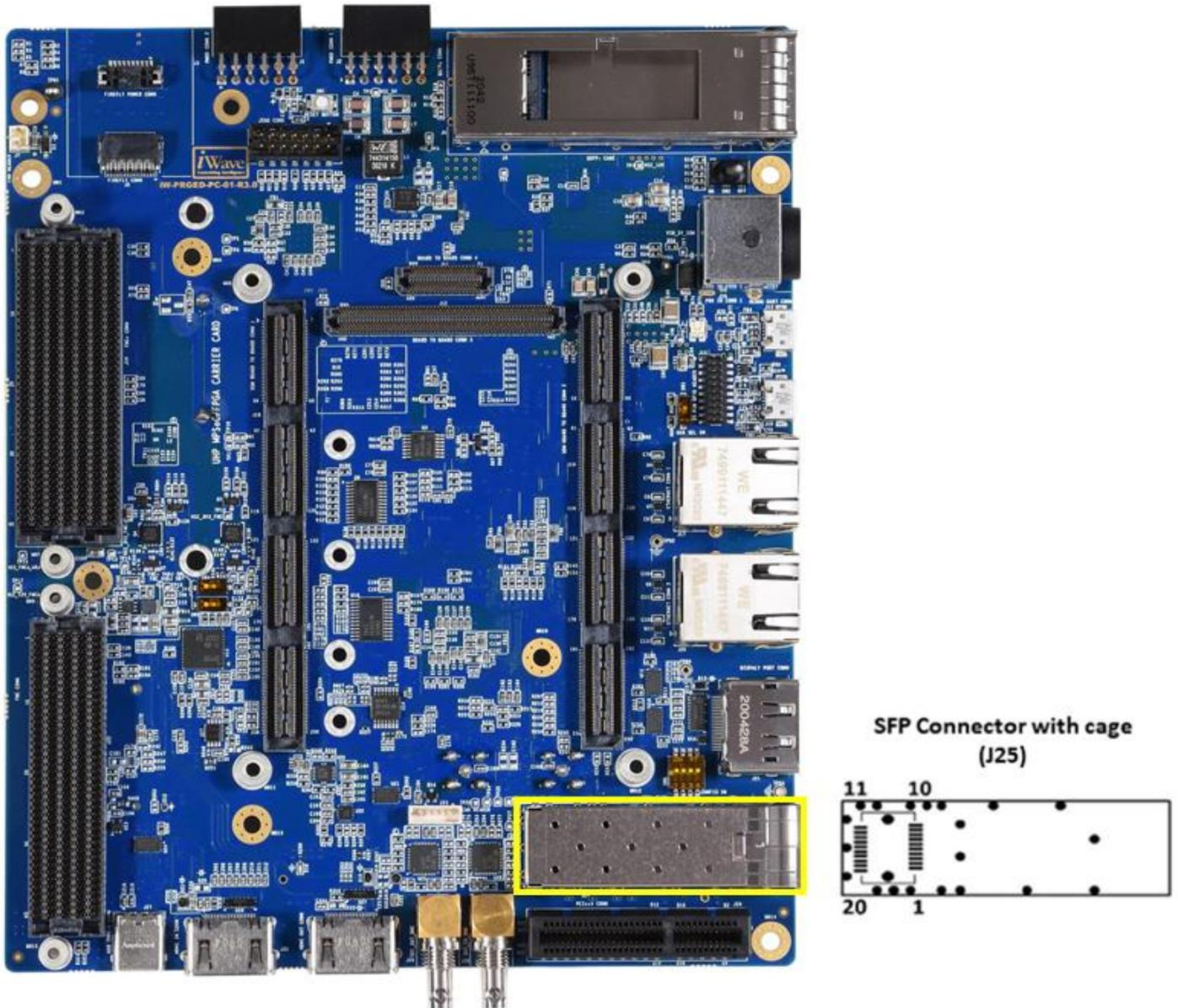
Figure 16: SFP+ Connector with Cage
