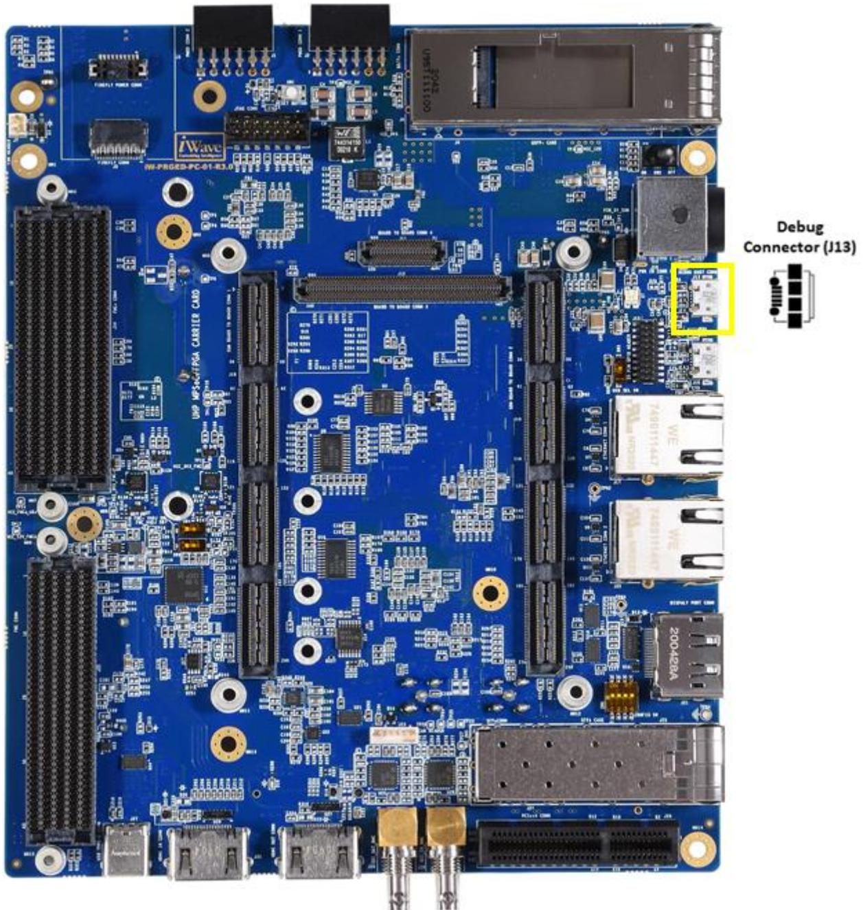
Figure 9: Debug UART Connector
