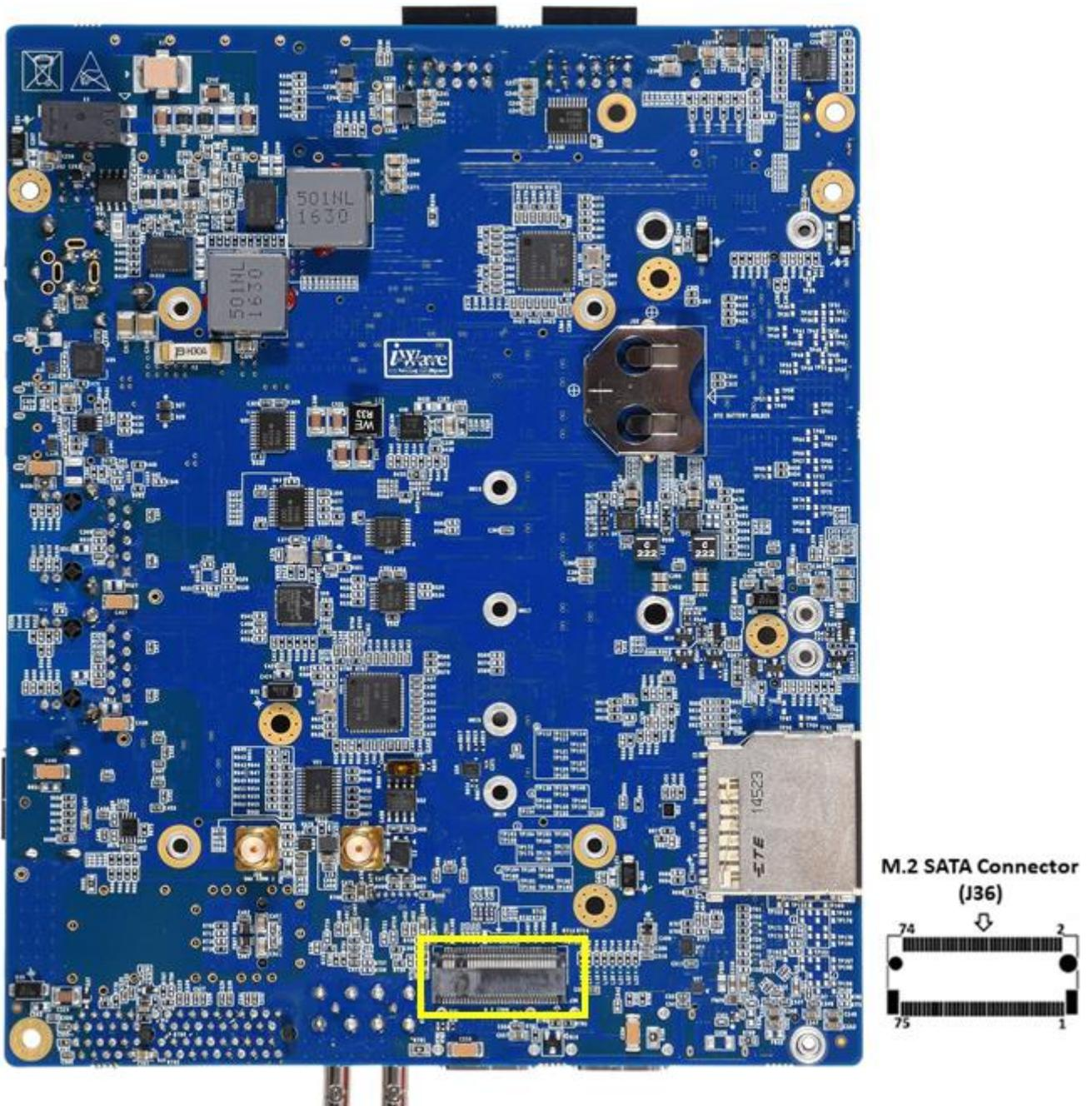
Figure 15: M.2 SATA Connector (Key M)
