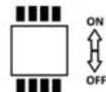
**Figure 11: Transceiver Lane Selection Switch**
