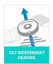
Allows for proper heading output when surface is uneven
