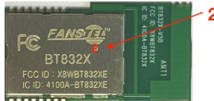
**BT832X-p and BT832XE-p:** All BT832X-p and BT832XE-p are new version devices. There is a “P” marking above the “X” or “XE” to indicate supporting of approtect.
