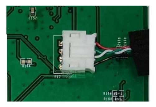
Figure 599: Capacitive Touch Connector
