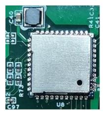
Figure 600: RTL8821CS WiFi/BT Module
