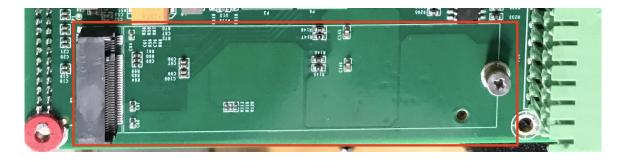
M.2 2280 Slot for PCI-E 3.0 x 2 NVME SSD
