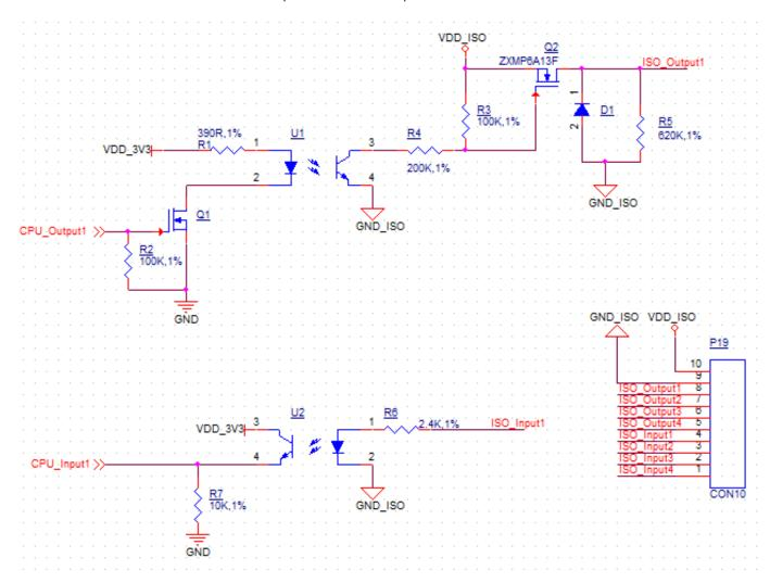
Isolated GPIO reduced schematic
