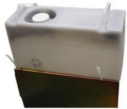
Figure 1: Chillers Reservoir with Algae Growth Along Top (the discolored areas)
