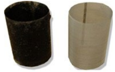
Figure 8: Chiller pump strainers – dirty and clean, respectively
