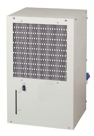
A Modular Cooling System (MCS) is a cost-effective and reliable alternative to refrigerated chillers for applications where precise temperature control and cooling below ambient temperature are not required. It consists of a high performance Boyd heat exchanger integrated with a fan, pump, and tank in a durable metal chassis.
