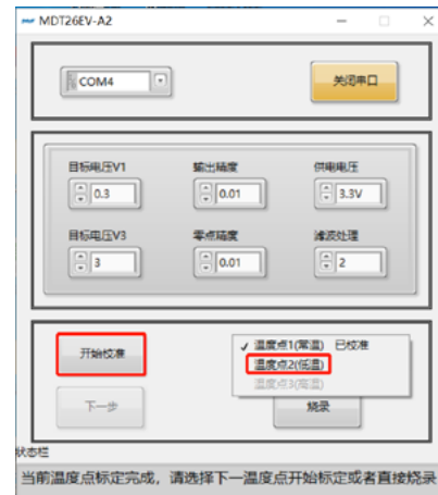
Figure 8.6 To calibrate at additional temperature
