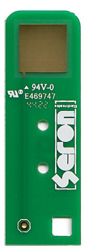
With a surface area of 1 cm<sup>2</sup>, SE.32 is ideal for energy material characterization. Coated with gold, they are chemically stable, biocompatible, and durable.
