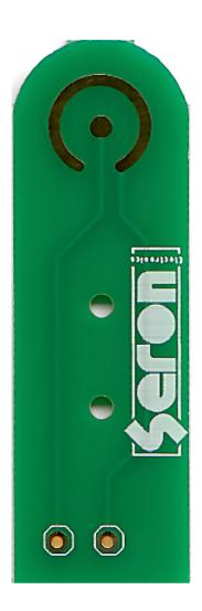
With a surface area of 1 cm<sup>2</sup>, SE.34 is ideal for biomaterial characterization, and touch/pressure sensor devices. Coated with gold, they are chemically stable, biocompatible, and durable.
