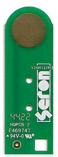
With a surface area of 1 cm<sup>2</sup>, SE.31 is ideal for energy material characterization. Coated with gold, they are chemically stable, biocompatible, and durable.
