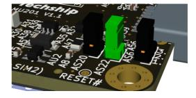
**NOTE** – Sierra Wireless EM9190, EM9191, EM7690 and EM9291 defaults to PCI Express data interface. To activate usage of USB2/USB3 data interface instead, assemble jumpers on pin 20 and pin 22 signal pin-headers.
