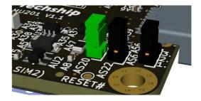
AS22/DS22 – pin-header, use 1.27mm jumper to pull M.2 socket pin 22 signal high with 1.8V DC.
