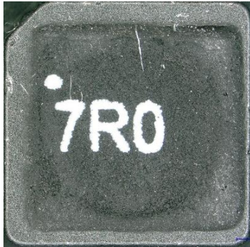
Marking with Pad Printing
