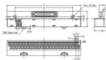
Note: There is only one DIN Track lock located in the center of the terminal block for a 20-pole Unit.
