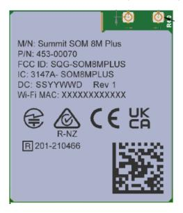
After this PCN, both the Wi-Fi MAC and ELAN MAC with B0FB15 OUI will be laser-etched on the RF shield and embedded in the 2D barcode.
