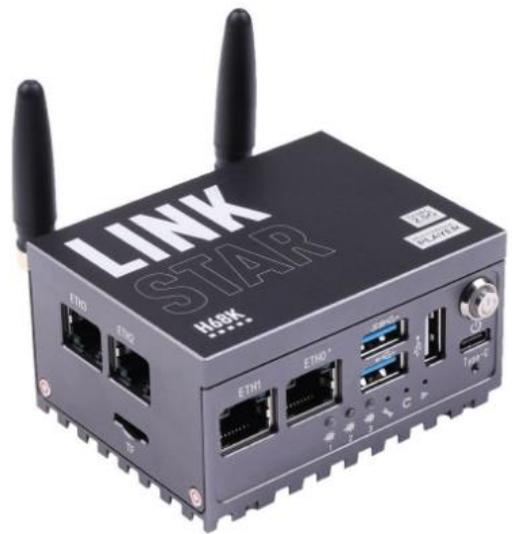
**LinkStar-H68K-1432 Router with Wi-Fi 6, 4GB RAM & 32GB eMMC, dual-2.5G and dual-1G Ethernet, 4K output, Pre-installed Android 11, Ubuntu 20.04 and OpenWRT support, Home Assistant**
