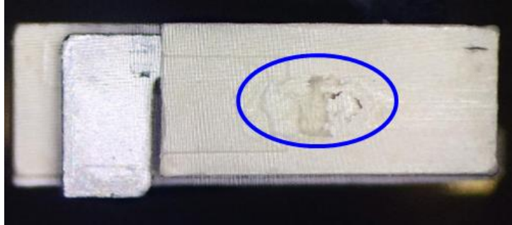
Gate location - side position of resin core.
