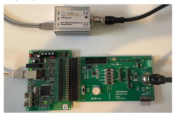
Do **NOT** close J2 when using the SSC Communication Board at the same time as powering the board via the IO-Link line!
