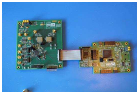
Figure 2: EV9830 Host Port Connected to HB9830
